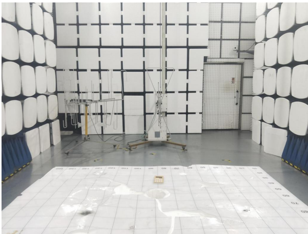
Test Setup Photo of Radiated Measurement (30MHz~1GHz)
