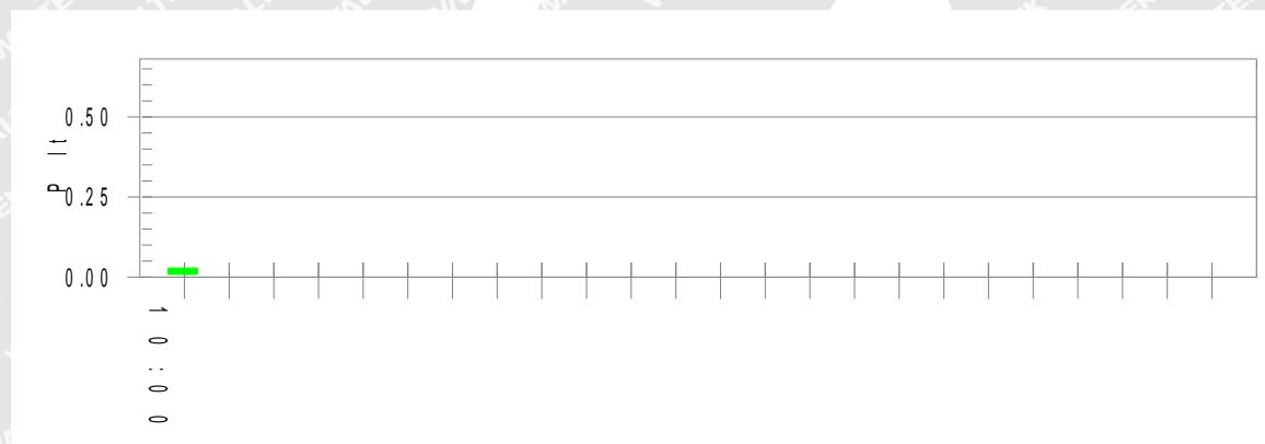
**Parameter values recorded during the test:****Vrms at the end of test (Volt): 229.99****T-max (mS): 0****Highest dc (%): 0.00****Highest dmax (%): 0.00****Highest Pst (10 min. period): 0.064****Highest Plt (2 hr. period): 0.028****Test limit (mS): 500.0****Test limit (%): 3.30****Test limit (%): 4.00****Test limit: 1.000****Test limit: 0.650**
