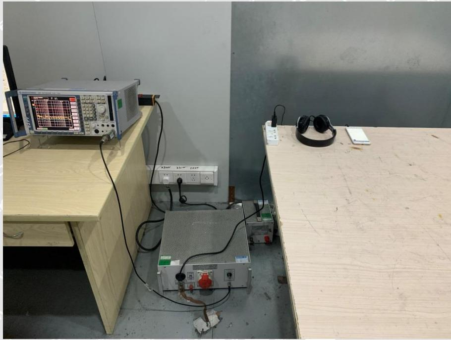
Radiation Emission Test View (Below 1GHz)
