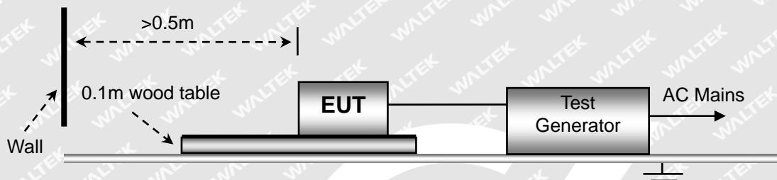
For Signal or Telecommunication Ports:
