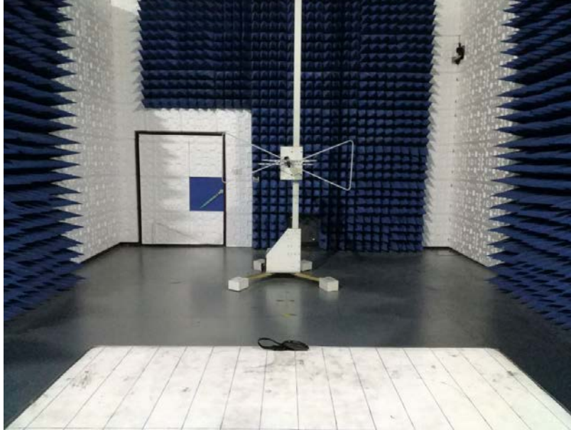
EN 61000-6-3 RADIATED EMISSION TEST SETUP
