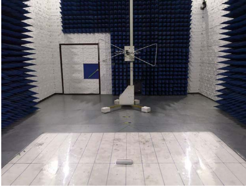
EN 55015 RADIATED EMISSION TEST SETUP
